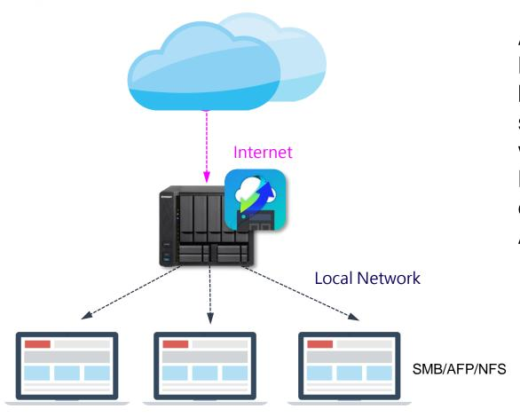
After connecting public and private cloud with **HybridMount** as a gateway, the transferring between cloud drives and the NAS is simplified, and the user could access files with fast local network.
